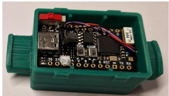
Figure 2: Device in enclosure - top view
