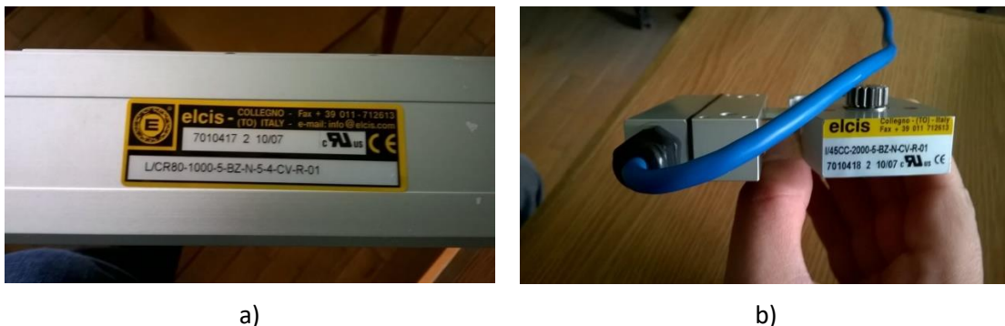
Figure 3: Ruler (a) and counter (b) of the ELCIS displacement transducer
